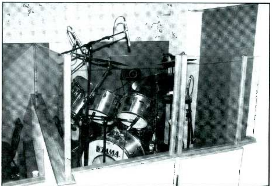
Figure 2. In a church setting, baffle-enclose the drums.
